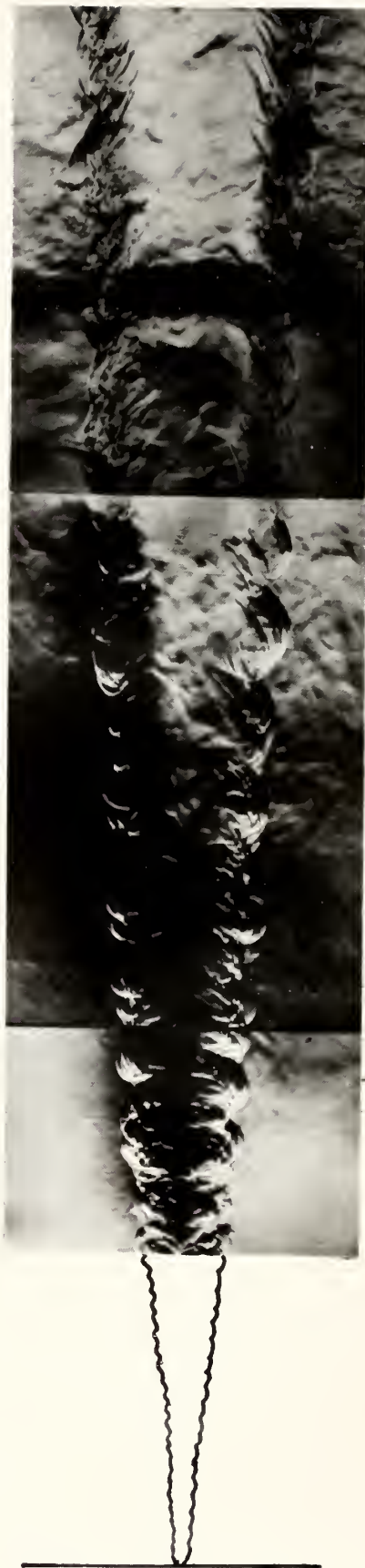
Figure 12. Composite Photograph of Flame Spreading from 1/8 inch Diameter Flameholder; \phi = 1.0 , 300 ft/sec Mixture Velocity
